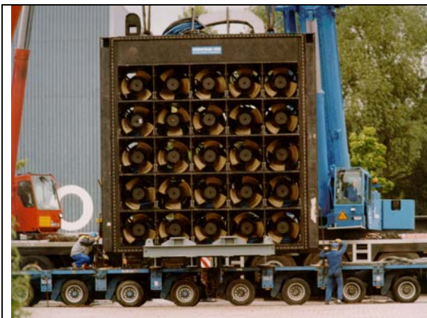
Picture 1: 5 x 5 Unit Module of Freudenau HYDROMATRIX® plant
