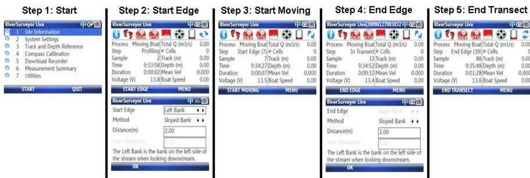
Figure 5. Five steps in completing a discharge measurement
