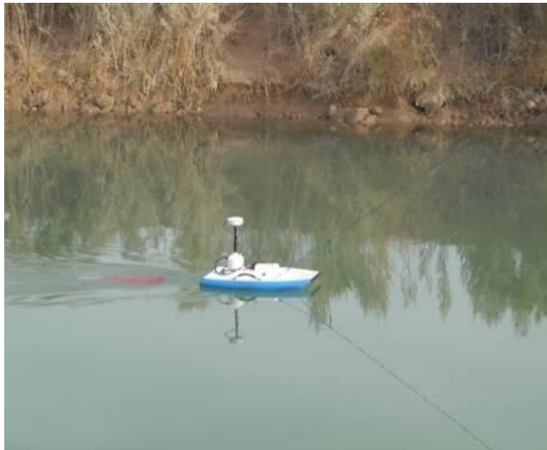
Figure 4. SonTek RiverSurveyor assembled on SonTek Hydroboard
