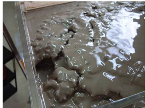
Surface cracking when irrigation is applied (top view)
