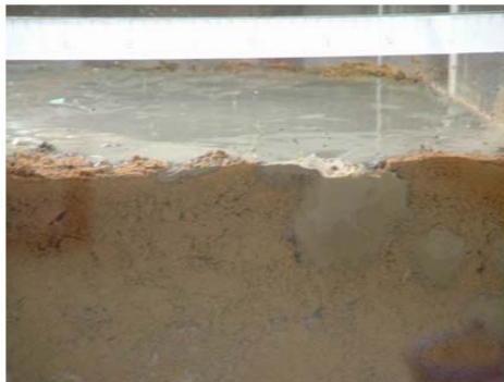
Surface cracking when irrigation is applied (side view)
