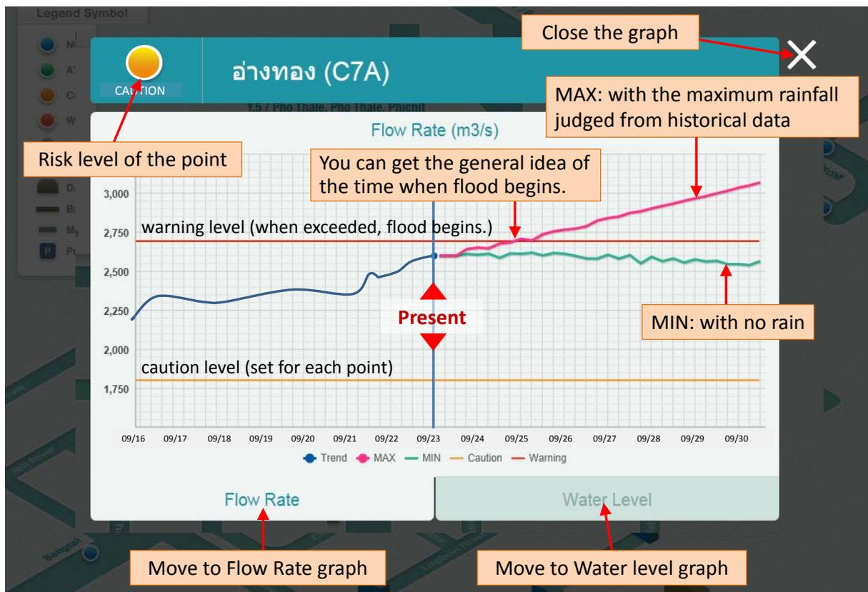
**Fig. 8** River Flow Rate Transition and Forecast Graph
