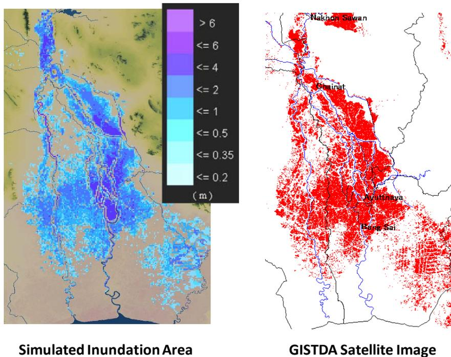
**Fig. 4** Satellite Image with Inundation Depth Information?
