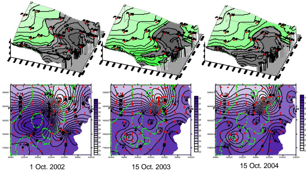
**Fig. 14** Flood map and GWL contour in high flood period
