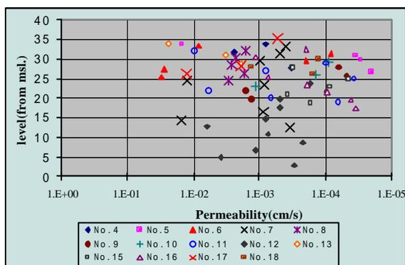
**Fig. 8** Results of in-situ permeability testing at observation well points
