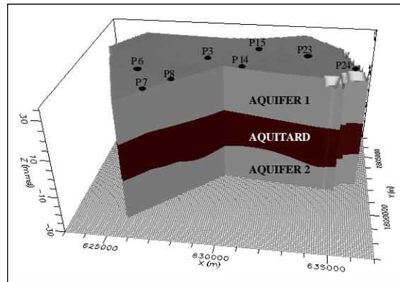
**Fig. 20** The cross section of hydrogeological condition in study area
