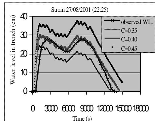
**Fig. 28** Simulation result of storm, 27 August 2001
