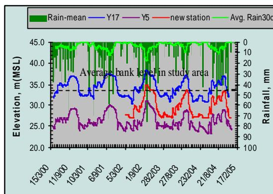
**Fig. 9** Daily water levels of the Yom River at Y5, Y17 and the new station in study area
