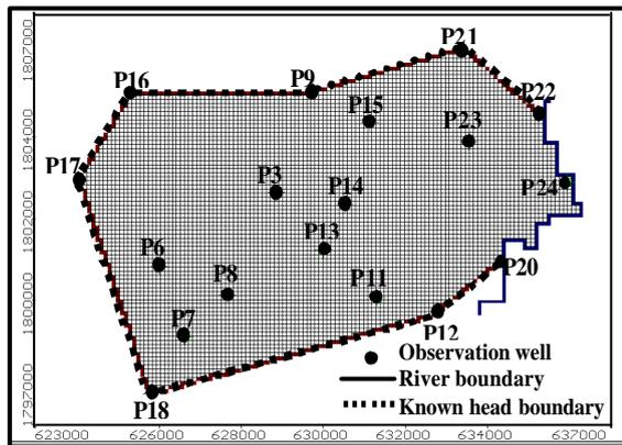
**Fig. 19** The model domain and boundary Condition
