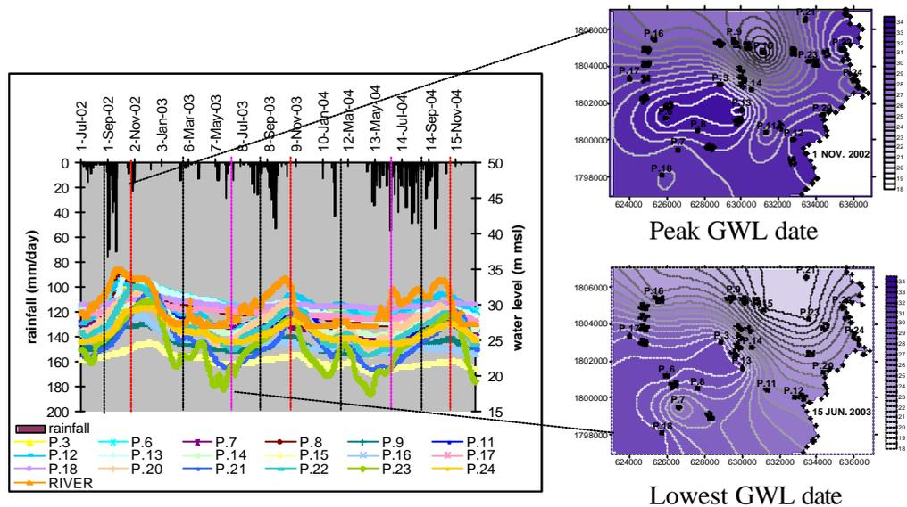
**Fig. 11** Rainfall, observed groundwater, Yom river water level and GWL contour map.
