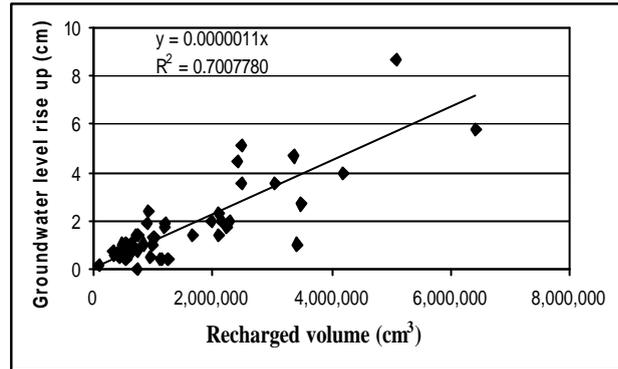
**Fig.30** Relationship between recharged volume and groundwater level rise up.
