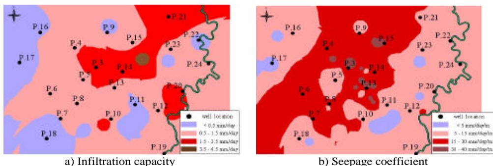
**Fig 10** The distribution map of infiltration capacity and seepage coefficient
