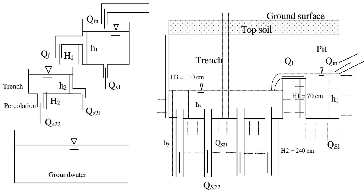
**Fig.26** The concept of simulation using tank model concept
