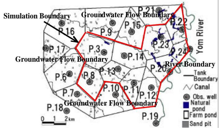
**Fig. 18** Thiessen polygon, simulation boundary and boundary condition
