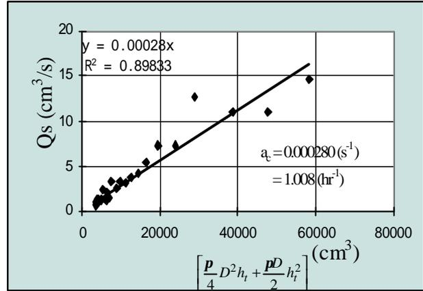
**Fig. 25** The seepage capacity coefficient of percolation well no.1
