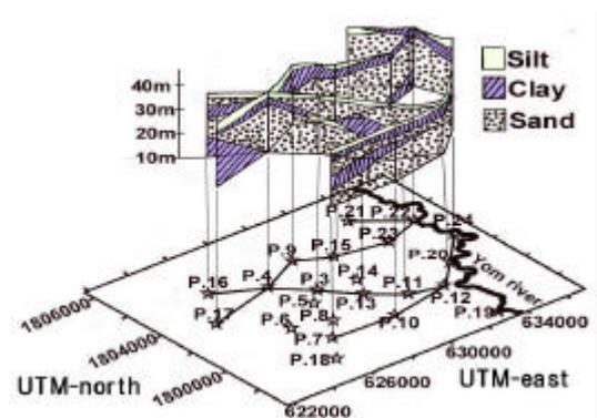
**Fig. 7** Soil log constructions in 3-D
